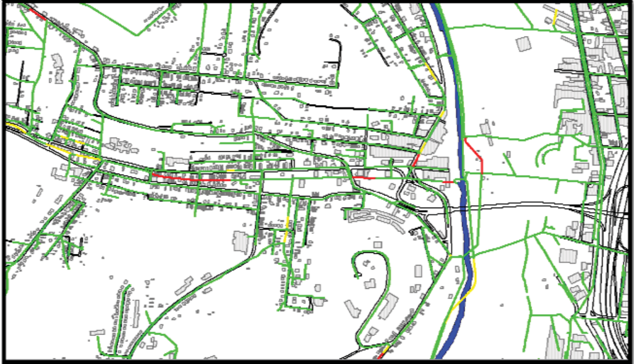
Figure 5.3: Camp Washington Area Critical Sewers
